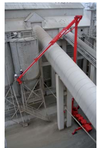
Figure 2: Elevating platform LEO for exceptional height and distances
