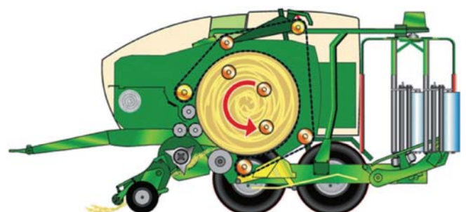
Figure 3: Schematic of a winding unit on a round bale press
