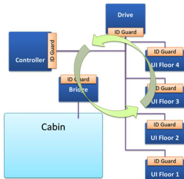
Figure 2: With ID guard protection, all devices protect each other
