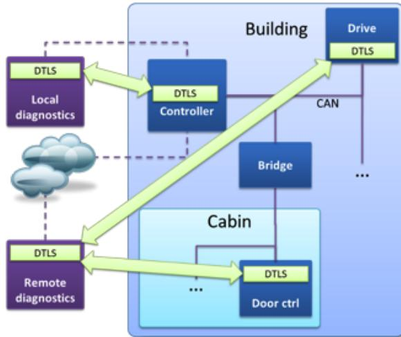
Figure 4: End-to-end security between individual devices using DTLS
