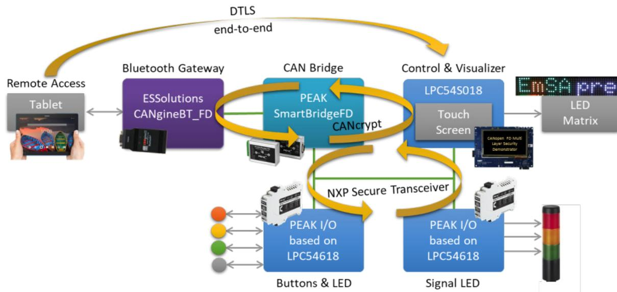
Figure 7: Demonstrator setup
