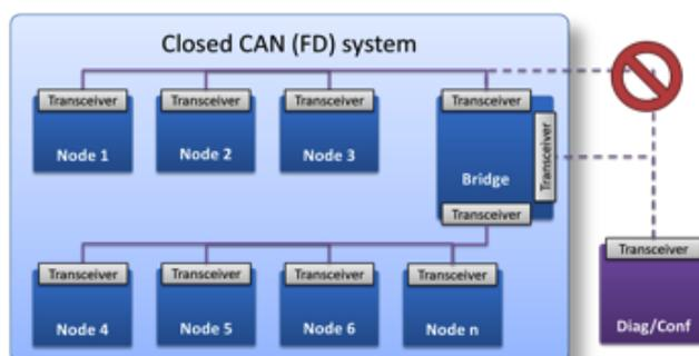
Figure 5: Temporary devices should not be allowed direct access to a CAN domain
