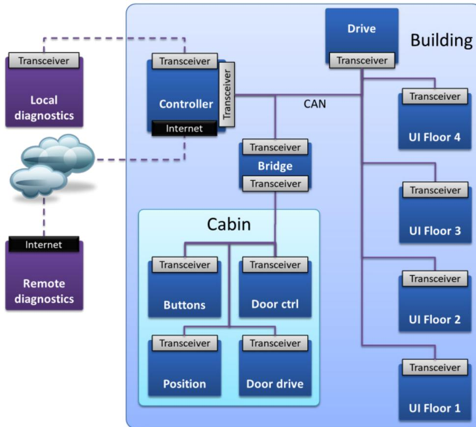
Figure 1: An elevator system with local and remote access for maintenance/diagnostics
