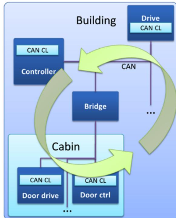
*Figure 3: Using a CAN cryptographic layer, devices can be securely grouped and authenticate messages*
