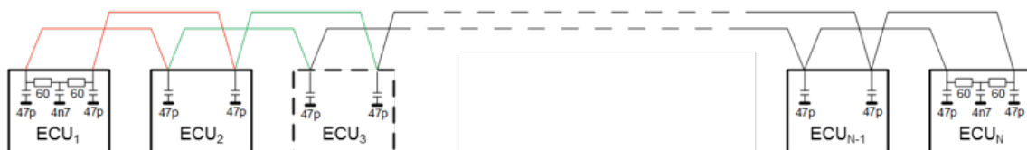
Figure 4: Example of a “ringing optimized” topology
