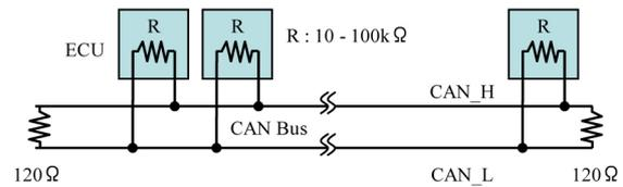
Figure 1: Physical layer of CAN FD
