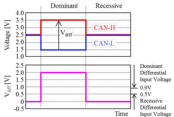
Figure 2: CAN FD typical voltage waveform
