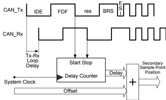
Figure 4: Loop Delay Measurement
