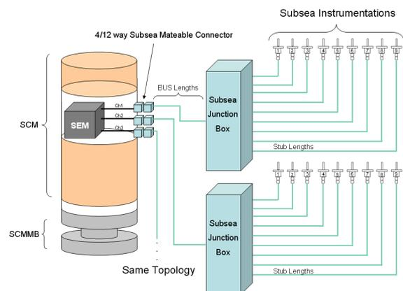
Figure 1: Typical Subsea CAN Topology
