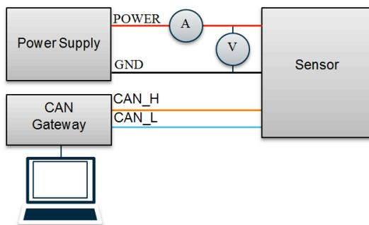
Figure 6: Power Consumption Setup
