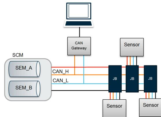
Figure 4: Subsea Control System Integration Setup
