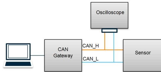
Figure 3: Single Sensor Test
