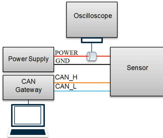
Figure 5: Inrush Current Setup
