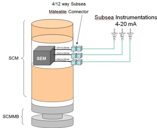
Figure 2: Typical Subsea 4-20mA Topology
