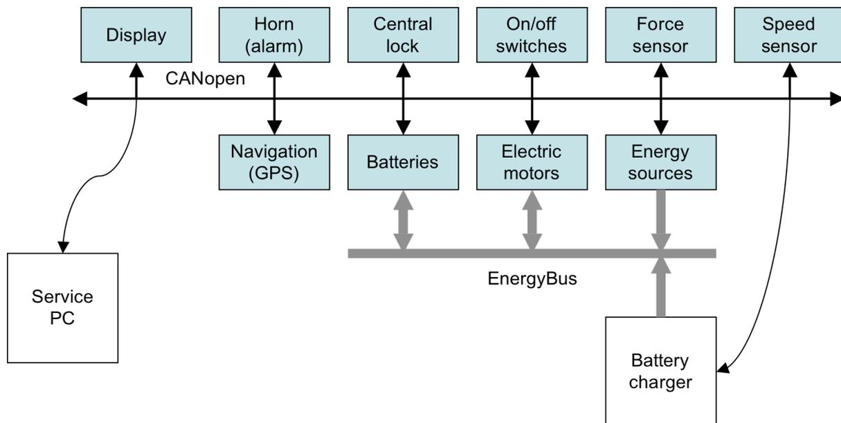
Fig.1: Possible system architecture in an LEV (e.g. Pedelec)
