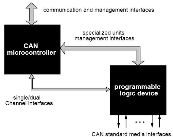
**Figure 2 CANELY Hardware Architecture**
