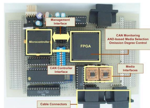
**Figure 3 CANELY Prototype**
