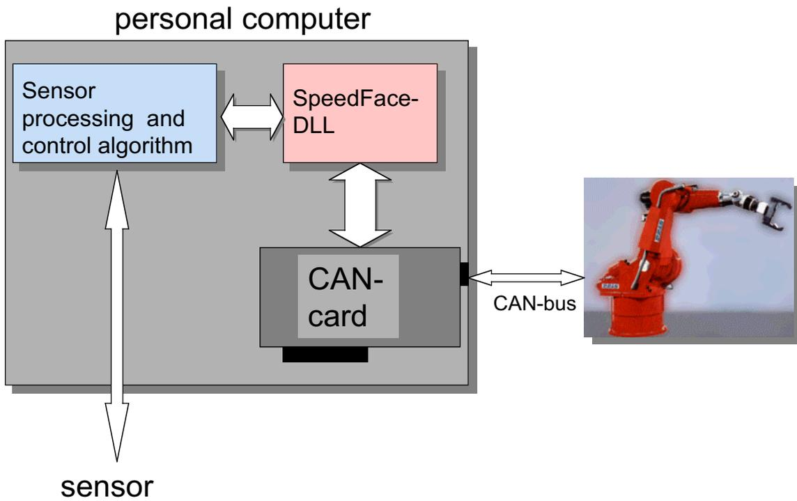
Figure 1: configuration of the link
