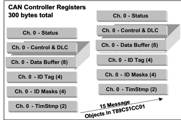
The controller also includes a 16-bit time stamp timer. Each transmit messages and receive messages can be time stamped. This feature can be used for instance to synchronize clock between a charger and a battery
