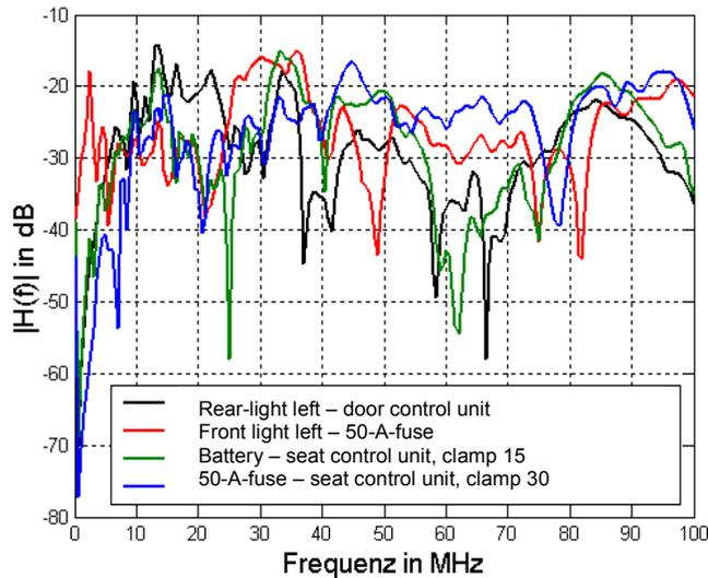
Fig.2: transfer function of standard on-board network (without modifications)
