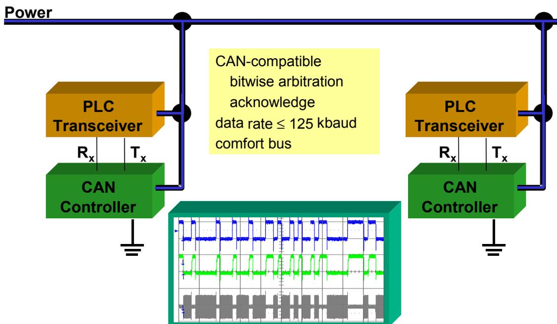
Fig.5: block scheme CAN-PLC-bus
