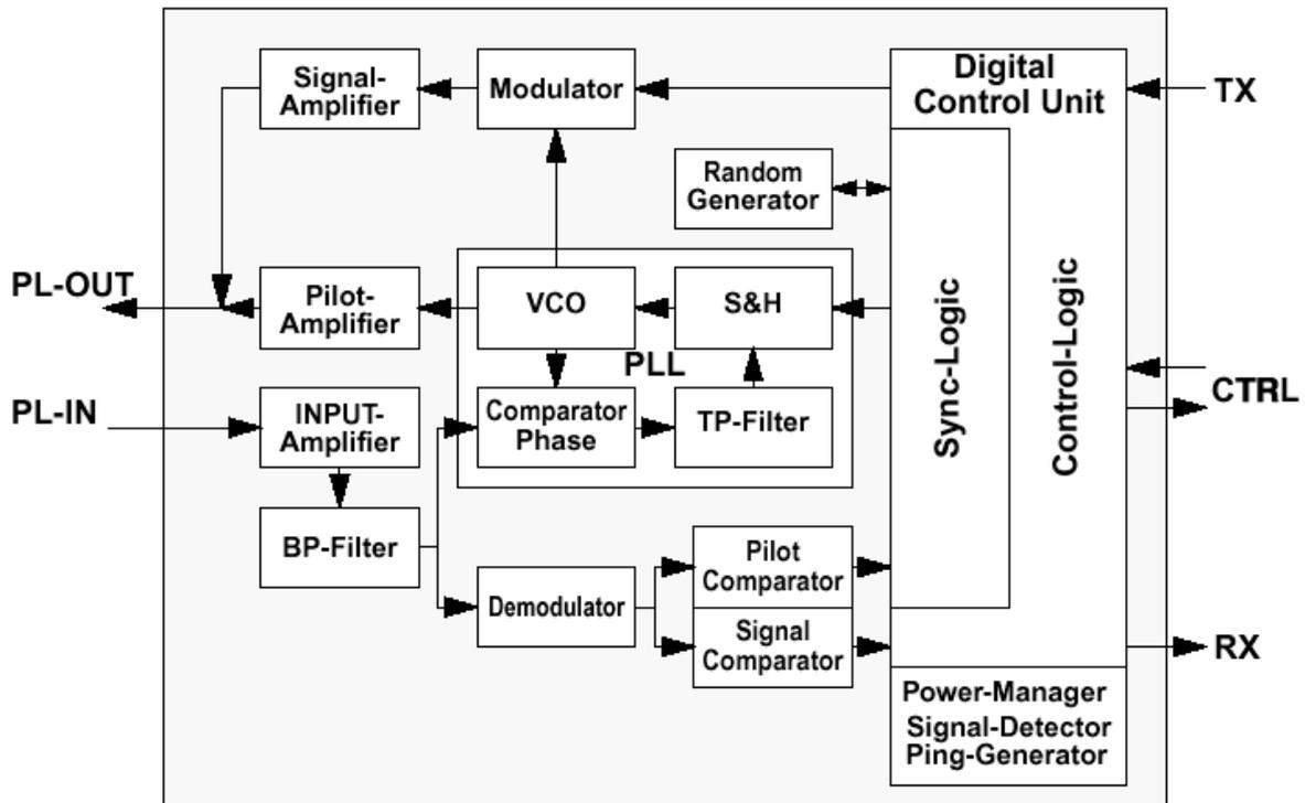
Fig.6: block diagram "one-frequency"-transceiver
