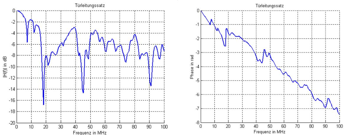
Fig.4: transfer function of door line harness (terminated with 150 Ohm)
