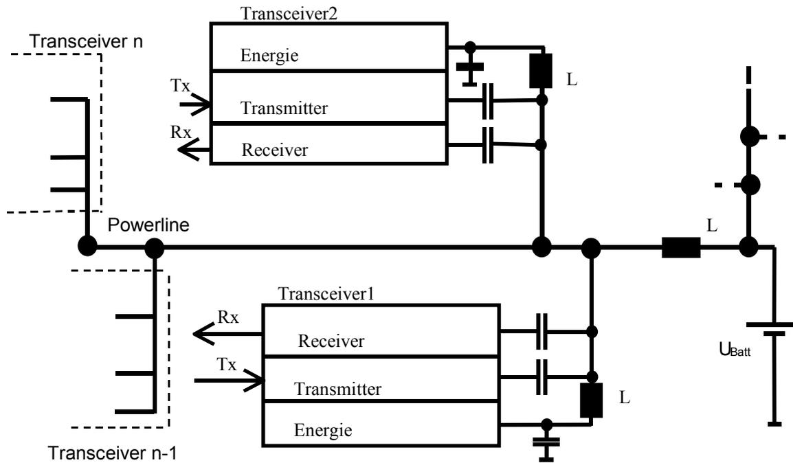
Fig.3: architecture of low-frequency PLC-system
