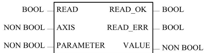
This function block reads data from the axis. PARAMETER defines the type of data requested. The way of addressing and the definition of Values are proprietary (if no standardization is made).
