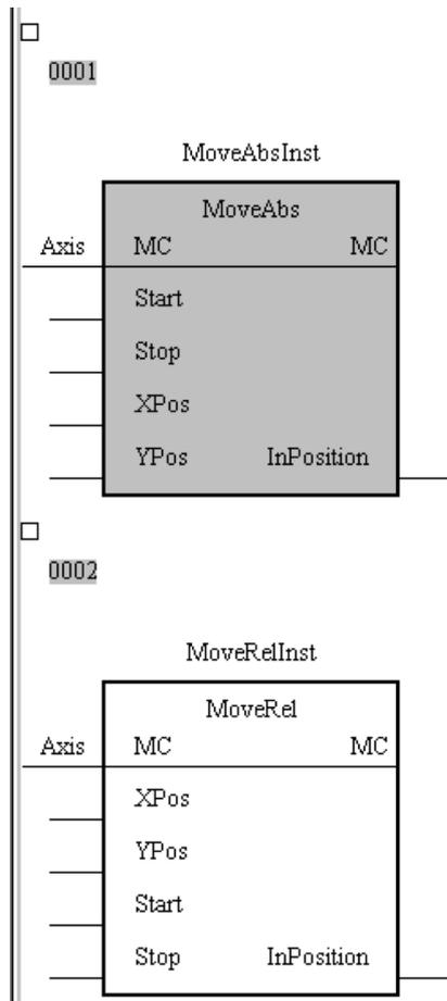
Instantiate the axis (Axis), and the MC functionblocks (MoveRelInst, MoveAbsInst).
