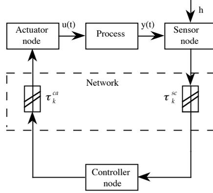
Fig. 1. Control system loop.
