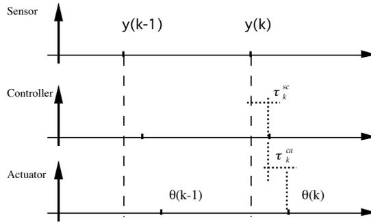
Fig. 8. Timing problems in the controlled system.
