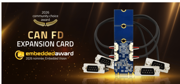
Figure 2: Awarded M.2 module with four CAN FD ports (Source: Cervoz)
